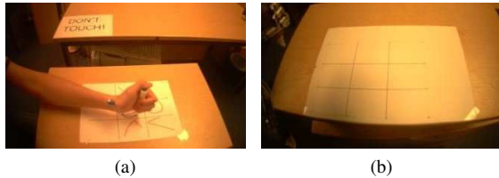
Fig. 3: Environmental setup for Experiment B. (a) shows an instance of the demonstrator drawing a circle in a cell of the A4-sized grid. The iCub was expected to play the game in scene (b), where the grid is 20% smaller, rotated and 20cm above that in (a).
