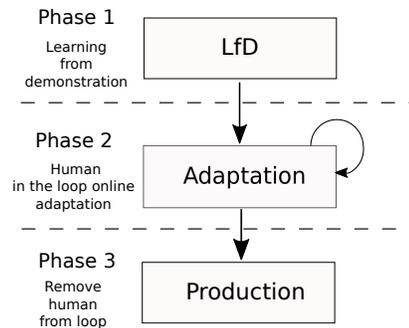
**Figure 1. Proposed three-stage LfD method. Adaptation phase is iterative with human corrections until high precision and accuracy is achieved.**
